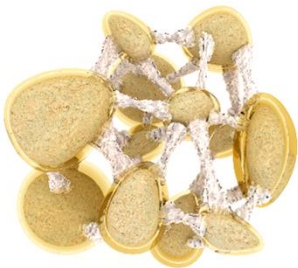
Figure 1. Calcium carbonate deposition among the soil contaminated grains
