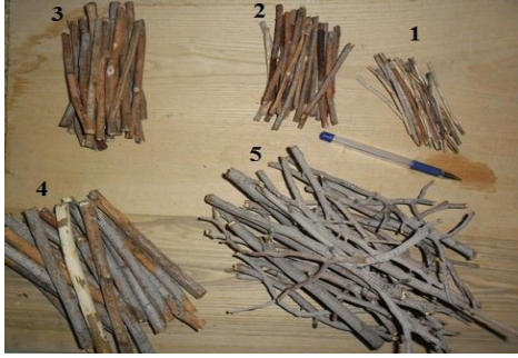
Fig.2. model debris including, trunks (from 1 to 4) and rootstocks (5)
