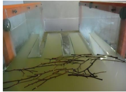
Fig.3. A view of blockage the rootstock in PKW
