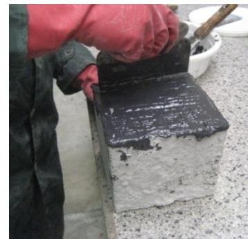
Fig. 2- Application of the glue to the CFRP sheets.
