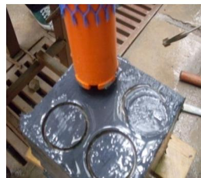
Fig. 3- Partial cores for Twist-off testing.
