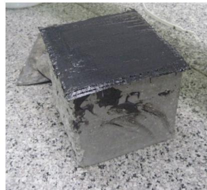
Fig. 1- Sticking the CFRP sheets to the glued surface of the concrete.
