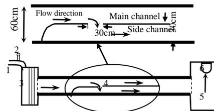
Figure 1. Schematic view of a laboratory flume
