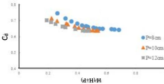
Figure 4. Variation of laboratory discharge coefficient relative to  $H/(H+P)$
