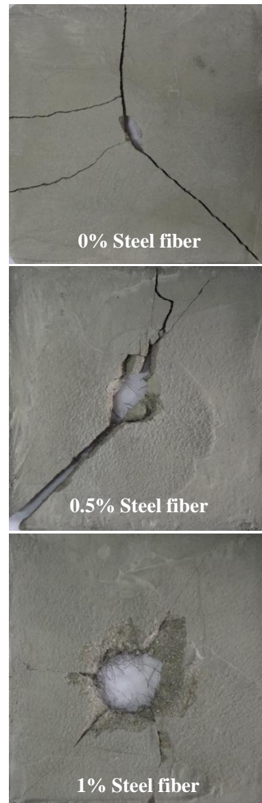
Fig. 3. Failure mode in plain concrete slabs and RC slabs under drop weight impact
