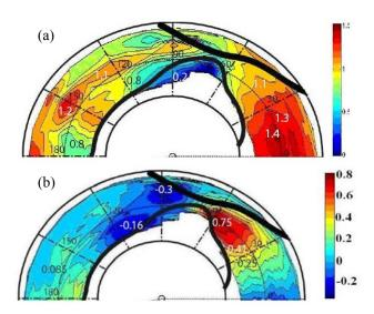
Fig 2. Experimental results: (a) Longitudinal depth-averaged velocity (Us/U), (b) Transversal depth-averaged velocity (Un/U)
