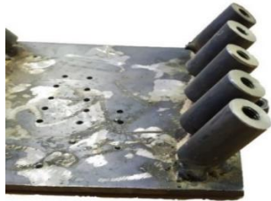
Figure 1. A view of the couplers connected to the pile
