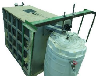
Figure 2. The sand container along with the frame and water tank
