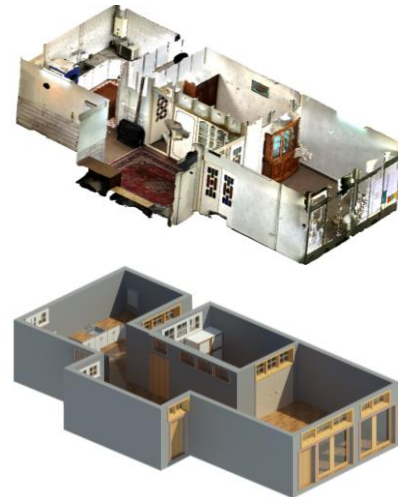
Figure 3, Preparing a valid and realistic building information model using a 2D map and 3D point cloud information
