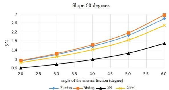
Fig. 5 The chart of coefficient of confidence changes based on the values of the internal friction angle in the soil with a gradient of 60° and adhesion of 3 tons per square meter and specific gravity of 2 tons per cubic meter
