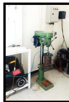
Figure 1. The new laboratory machine to determine soil abrasivity
